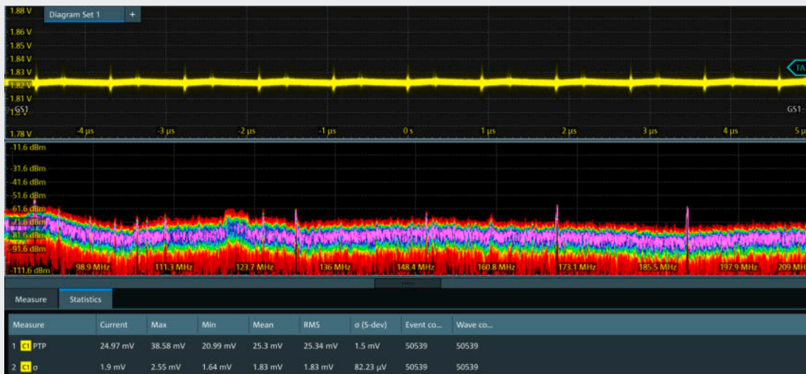
Using spectrum analysis with time gating to effectively find coupled sources that contribute to power rail noise
